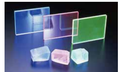
Functional fluorescent glass, which efficiently converts faint light into visible light
